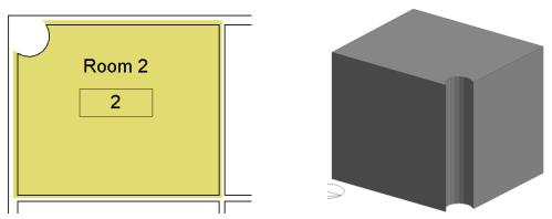
The Revit model and the corresponding DesignBuilder model before the change, with the column being a room bounding element.
