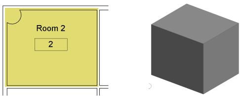
The Revit room and the corresponding DesignBuilder zone after de-selecting the column as a room bounding element. The DesignBuilder model following the fix will be more accurate and because there are less surfaces, calculations will run faster.
