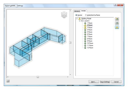
You can use the Export gbXML dialog to visually detect gaps between zones in the analytical model. You should generally aim to avoid gaps in the analytical model to ensure correct zone volumes and adjacencies in the DesignBuilder model. For example in the model below you can see gaps (shown in white) between the 3 floors of the model.
