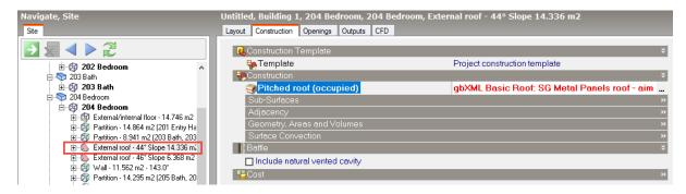
The equivalent settings in Revit can be checked as follows. Navigating to the equivalent roof surface in Revit you can see that the **Basic Roof SG Metal Panels roof** has been set:
