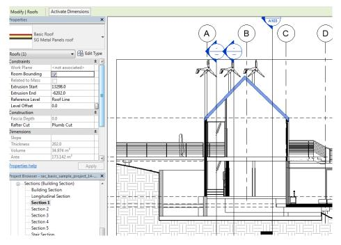
You should see that in this Revit assembly is made up of four material layers. However, the thermal properties for **Roofing – Metal Standing Seam** and **Wood – Furring** have not been set up:
