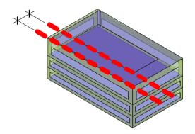
The core of a building has heating and cooling loads that differ from the perimeter because it is not directly exposed to external weather conditions or daylight through windows. A typical perimeter zone depth is 12-15 feet (4-5 m).
