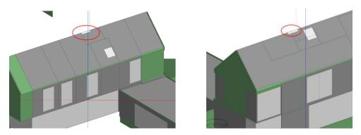
**Note**: these erroneous windows are included in the Revit Analytical model and hence the gbXML generated by Revit.
