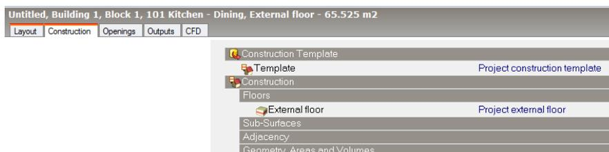
To understand the reason for this it is necessary to check the settings in the Revit model. Looking at the thermal properties for the Revit constructions: **Floor: Generic 150mm**, which is assigned to this floor in Revit, you can see that the thermal properties have not been completed in the Revit example model:
